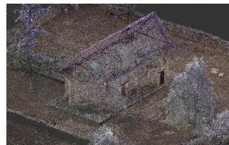
Figure 15: Point - Cloud Model of Asinou Church.
